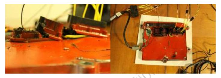
The leading four pin connector and front seventy-two pin connector are the most at risk, but the rearmost seventy-two pin connector is not immune. In this case, the housing of the four pin connector was destroyed and had to be removed to access the pins. Also, a clamp was needed to push the rearmost seventy-two pin connector back onto the circuit board. Once the connector was back in contact with the circuit board, jumpers were installed to achieve communications.
