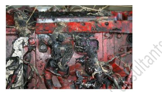
The ECM was damaged. The cab wiring harness was pulled completely out of the connector. The engine harness was secured to its connector, but the connector was broken from the ECM housing.
